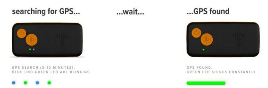
Activate tracking mode. Therefore push down the big PLAY button for 2 seconds.
